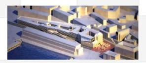
The Western Žabica Complex includes the construction of a new bus terminal near the old bus station. In addition to the construction of a new bus terminal, the project will include building of a public garage on 4 levels with 940 parking spaces, a shopping centre and business facilities.
